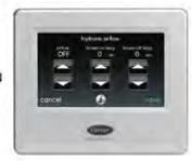
HYDRONIC AIRFLOW is the desired airflow during Hydronic Heating. The selectable airflows are OFF, 500 CFM, the minimum CFM, up to 400 CFM/ton cooling in 50 CFM increments. The factory default is 350 CFM/ton cooling airflow. The OFF selection does not turn off airflow if the heat pump is in the defrost mod.
