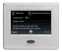
The second ZONING CHECKOUT is the Sensor/Damper Check that allows the installer to check each zone damper for operation and to confirm that the correct zone sensor is wired to a particular zone.
