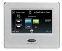
Since there is no bypass damper, the Zone Airflow Limit check will allow the installer to assess the airflow noise generated by the system. The Zoned Communicating Control provides the maximum amount of airflow to each zone individually. The technician can then modify the maximum amount of airflow to each zone by changing the Zone Airflow Limit setting.
