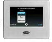
The G TERMINAL option is a feature used only on fan coils and furnaces with the control system. The indoor unit control board used in the furnace and fan coil includes functionality to the "G" terminal when the Communicating Control system is used. By the addition of a relay or switch with its contacts connected between the R and the G terminal on the board, a change of state of the switch will send a signal to the board to perform a predetermined function.
