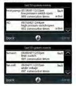
If the UI indicates an active system malfunction, it is a malfunction that is currently in effect. Each entry has the time and date from the most recent incident. The service technician should record the current date before checking and logging the last 10 system events. These events are stored in the memory of the Touch Control and are resettable the RESETABLE FAULTS selection.
