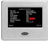
If a mistake is made on the start-up screen or a change is made to some of the accessories in the system and you see that the EQUIPMENT SUMMARY does not match the system, here is how you get back to make the change to the system. Let's use the ventilator as an example and assume that the system does not contain a unit ventilator. Notice that in this example that YES appears after ventilator and you want to change that to NO.
