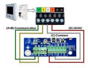
When working on a rooftop unit or outdoor unit of a split system with communicating controls and the UI is mounted and located indoors, it is time consuming operating the UI indoors then running outdoors to check unit operation. To overcome this, the communicating control has the ability to add a second UI outside wired into the outdoor unit board board.
