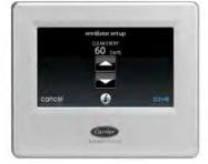
VENTILATOR will only be displayed in the ACCESSO-RY SETUP menu if a unit ventilator, an HRV or ERV, is installed into the system. The time interval to clean the ventilator pre-filter can be set so that the reminder is displayed at the UI. The time interval can be set from 60-days to 90, 120 or 180 days with the factory default value of 90-days.
