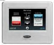
When the accessories filter SETUP is selected there will be three different types to select from. AIR FILTER, ELECTRONIC AIR CLEANER and AIR PURIFIER. An interval reminder can be set so that when the selected time has elapsed, the UI will display a message for the user indicating to change or clean the filter. This time can be set from one month to 18 months in one month increments. If the homeowner does not want this reminder display, NEVER is also a selection at this point.
