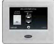
Ultra violet lights are displayed in the same manner. When a UV light is installed and YES is selected, a CHANGE INTERVAL time can be set from 6-months to 48-months, with 12-months set as the factory default value. And like the clean filter interval time and the humidifier change pad interval time elapsed, the UI will display a message to change the UV light.
