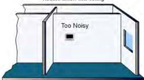
There may be a problem with some zones being too noisy due to excess airflow. In such cases, it is possible that the Zone Airflow Limit, configured at installation time, may be set too high. Perform an Airflow Limit Checkout procedure, reducing the airflow limit setting, if possible.
