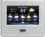
Weather can be viewed only after the WI-FI SETUP has been completed. Touch the WEATHER symbol to bring up a screen that displays VIEW WEATHER FORECAST and CHANGE CURRENT LOCATION. The first time that WEATHER is accessed the location must be identified. This is performed by touching CHANGE MY CURRENT LOCATION which will display a screen to enter your country and zip code for the United States or postal code for Canada.
