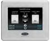
The same will happen with the HUMIDIFIER setup. If no humidifier is installed and NO is selected, the UI simply does not display an installed humidifier in EQUIPMENT SUMMARY. But, when a humidifier is installed and YES
