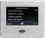
The SERVICE menus include EQUIPMENT SUMMA-RY, INSTALLATION, SETUP, CHECK OUT, SERVICE INFORMATION, SOFTWARE UPGRADE and DEAL-ER LOGO UPLOAD. REFRIGERANT CHARGING will also be displayed for the variable speed heat pump units.
