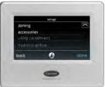
The SETUP Menu is tailored to the type of equipment that was identified during power-up. All setup parameters have been set at the factory with default values. For this reason a Quick Start can performed by entering a valid date/time and schedule as we explained earlier in this program.
