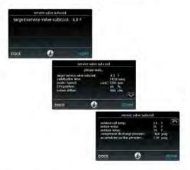
In order to add refrigerant charge the service technician will also have to select the line set length and the vapor line diameter as shown in the prior example.
