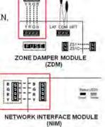
A ventilator may be connected to the system by wiring the ventilator directly to a ZDM in a zoned system, or a NIM in a non-zoned system. The system recognizes a ventilator is connected when the ventilator is wired to the YEL, RED, GRN, and BLU terminals of the ZDM or NIM, and the ventilator is powered.
