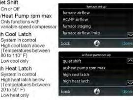
QUIET SHIFT can either be turned ON or OFF, the factory default position, will allow the outdoor fan to be turned on after the completion of the defrost cycle.
