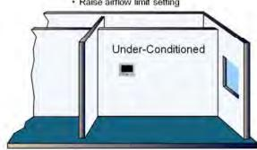
There may be a problem with some zones being underconditioned. That is, during cooling, the temperature of some zones is too warm and during heating, the temperature of some zones is too cool. In each case, there is a noticeable difference between the zone set point and its temperature. In such cases, it is possible that the Zone Airflow Limit, configured at installation time, may be set too low. Perform an Airflow Limit Checkout procedure, raising the airflow limit setting, if possible.
