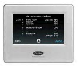
The ZONING CHECKOUT allows the user to perform a DUCT ASSESSMENT. This is the same check that is made during the initial start-up. The DUCT ASSESS-MENT will perform an airflow measurement on each zone and determine the relative size of each zone and the overall system damper leakage. This assessment will require approximately 1 minute for each zone in the system.
