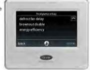
DEFROST FAN DELAY turns the outdoor unit fan on at the end of a defrost cycle for approximately 12 seconds to help reduce any nuisance refrigerant noise caused by reversing valve changing its internal position. This feature is only available on communicating heat pumps.
