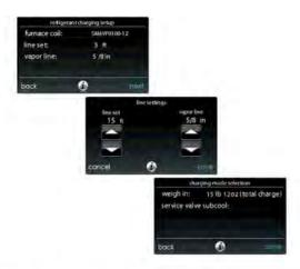
The refrigerant charging calculation takes into account the sizes of the indoor and outdoor units as well as the size, diameter and length, of the vapor line between the indoor and outdoor units. The liquid line size must be ¾-inch OD. If the liquid line and vapor line are different in their lengths, use the liquid line length for the length of the vapor line.
